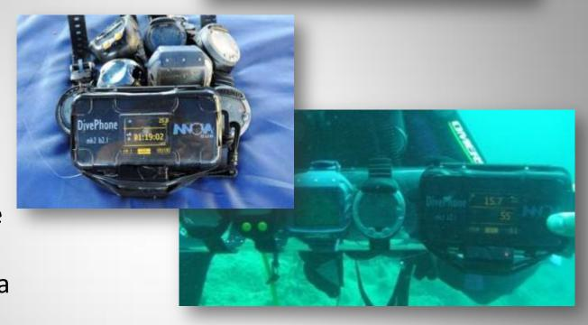
The Divephone is tested and benchmarked successfully with 7 existing dive computers in the market up to 42 m in open water conditions and in dry chamber.
